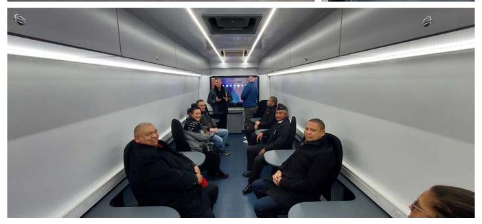
The workstation and kitchen area boasts the following fitted and secured neatly to allow optimum productivity including individual seating on fixed swivel office chairs, worktop, plugs, radios, printer, microwave, fridge/ freezer, LED lighting, inverter, LTE router, lockable cupboards and openable windows on either side of this space.
