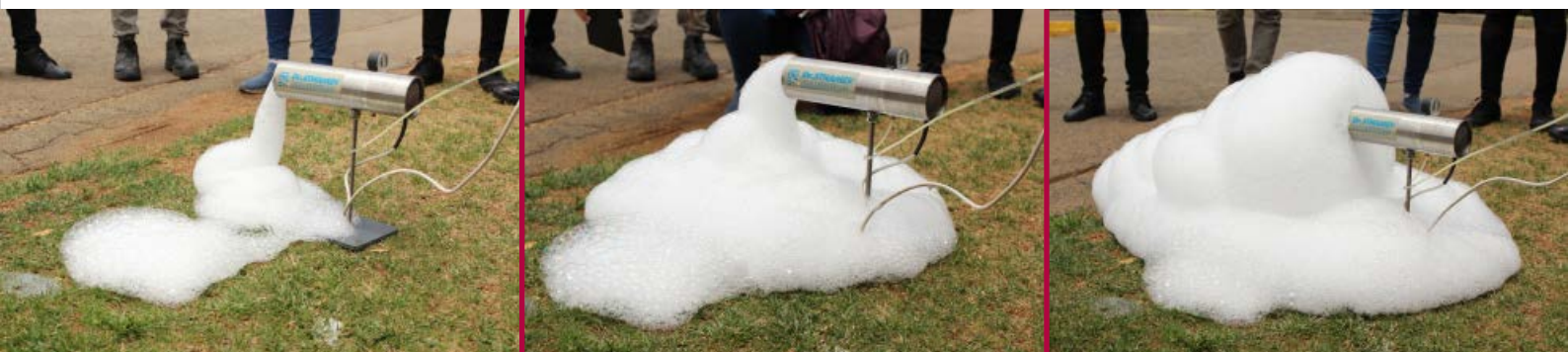
Demonstration with AECI's RLF 4 A class foam showing how the foam changes as you add or reduce air
