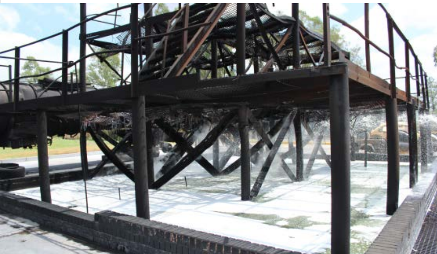
Firefighting demonstration with Fluorine free Vapurex 3% extinguishing an hydrocarbon fire (Avgas)
