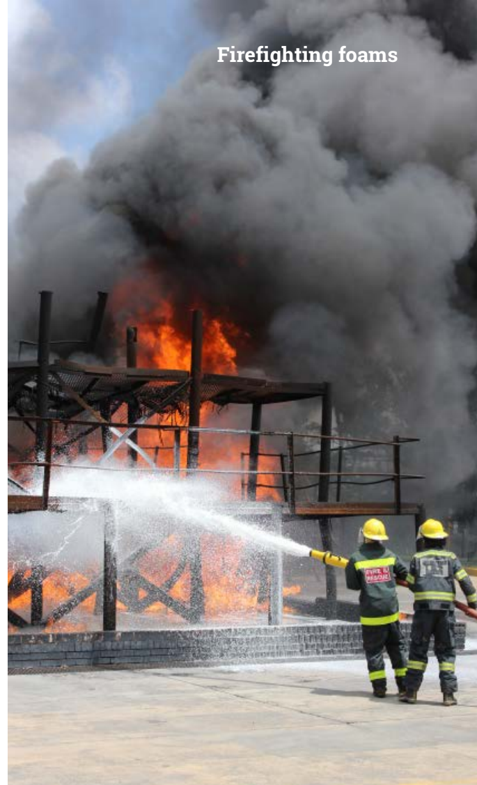
Firefighting demonstration with Fluorine free Vapurex 3% extinguishing an hydrocarbon fire (Avgas)
