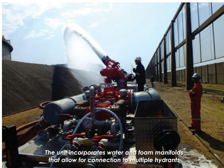
*The unit incorporates water and foam manifolds that allow for connection to multiple hydrants*
