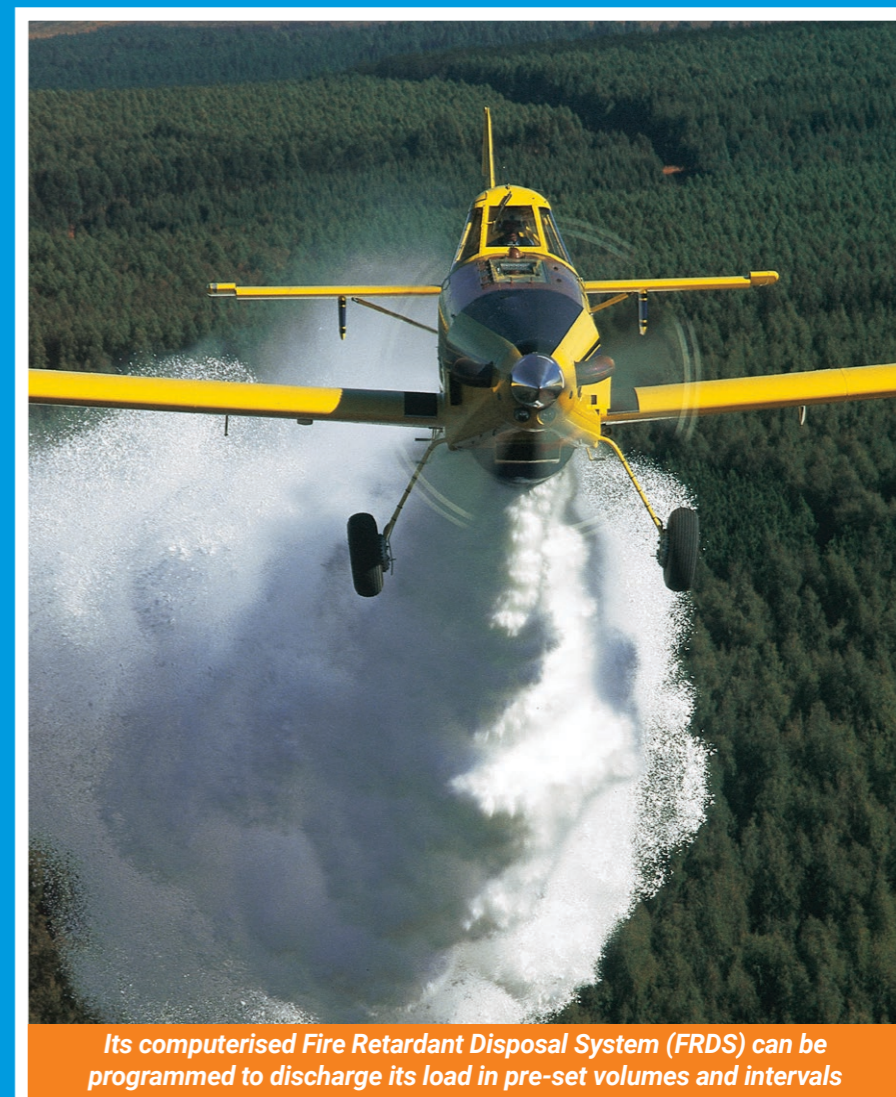
The AT 802 carries up to 3 104 litres of water, mixed with fire suppressants, reaching a cruising speed of 250km/h for rapid response to a fire line
