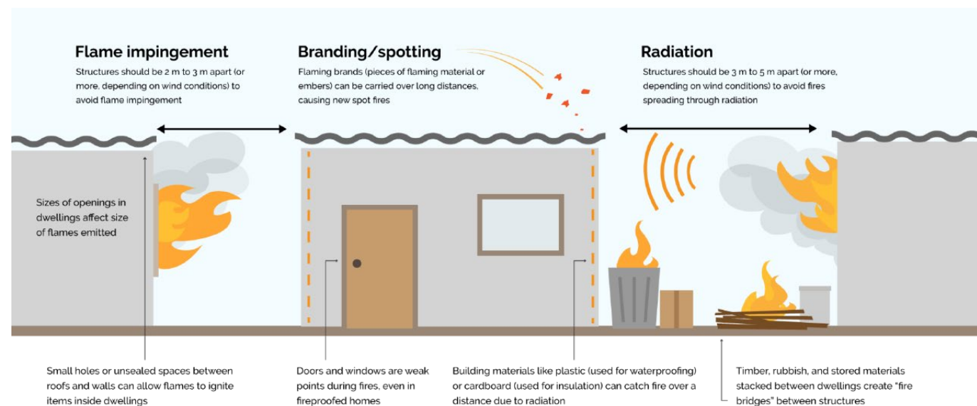
Illustration showing how informal dwellings catch fire from flame impingement (left), branding/spotting (middle) and radiation (right).
