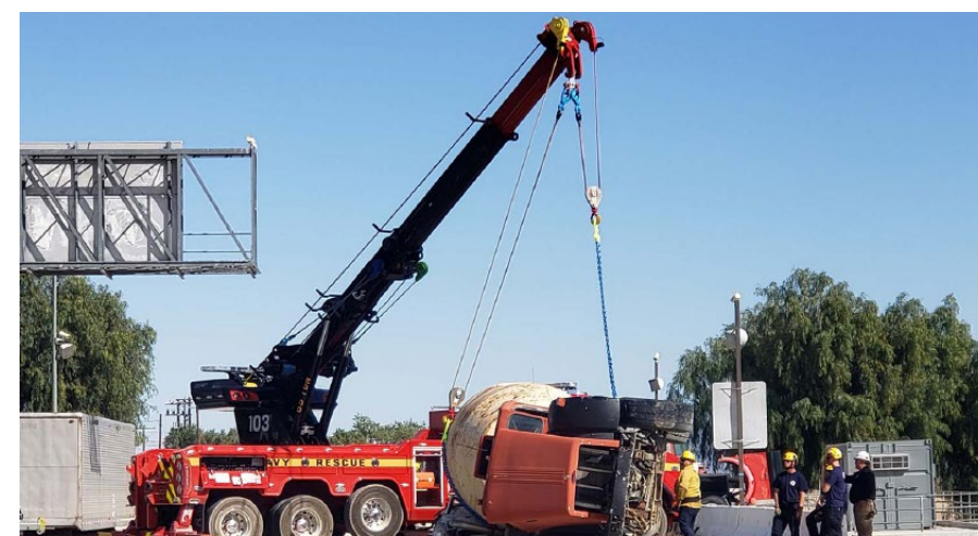
The tow truck's winching and lifting capabilities allow rescue teams to stabilise the damaged vehicle
