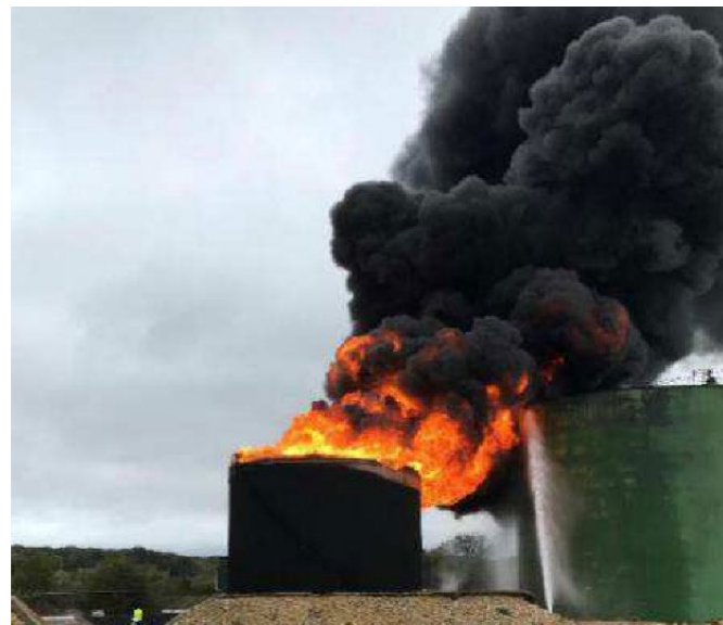
Tank used for Phase 1 of the LASTFIRE Fluorine Free Foam Testing
