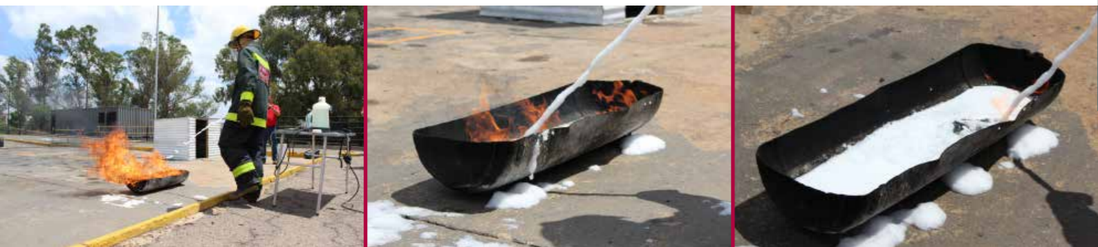
Demonstration extinguishing an alcohol fire using Fluorine Free alcohol resistant Vapurex AR 3X3 foam
