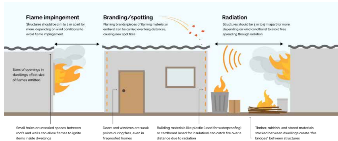
Illustration showing how informal dwellings catch fire from flame impingement (left), branding/spotting (middle) and radiation (right).
