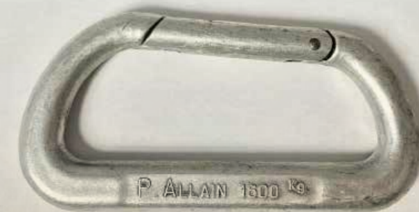
Pierre Allain aluminium carabiner, unknown exact date but likely between 1950s–1960s. Maker's mark "P. ALLAIN 1600KG" stamped on one side, reverse side stamped "BREVETE S.G.D.G." (sans garantie du gouvernement), which translates from French to "Patent without government guarantee." Richard K Irvin Collection
