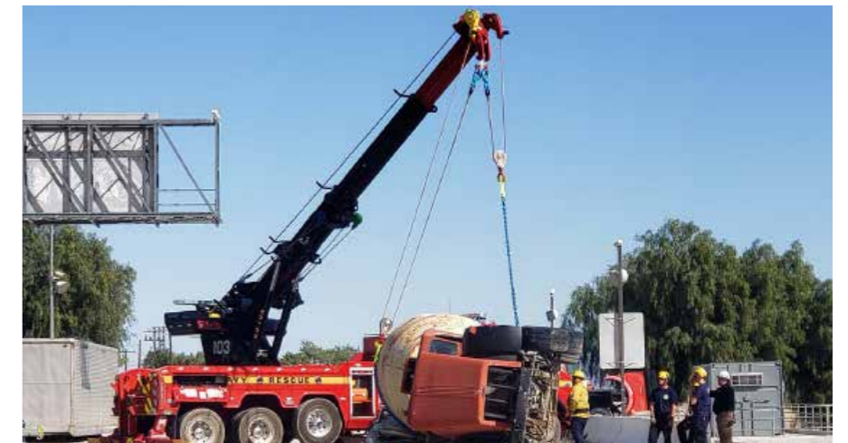
The tow truck's winching and lifting capabilities allow rescue teams to stabilise the damaged vehicle
