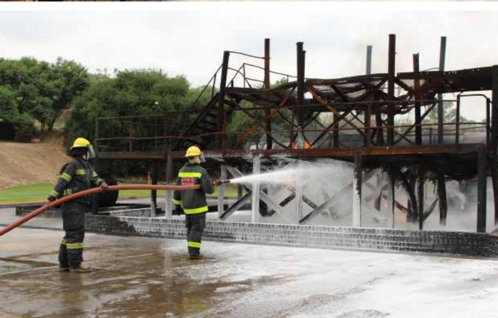
Demonstrating the effect of fighting the fire with Fluorinated foam AFFF 3%
