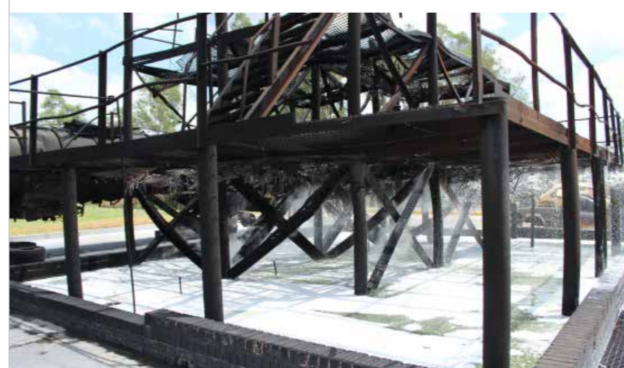
Firefighting demonstration with Fluorine free Vaporex 3% extinguishing an hydrocarbon fire (Avgas)
