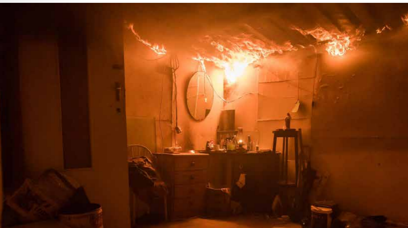
Following the ignition of a shack, the engulfing of the entire dwelling in flames or "flashover", happens extremely fast. Flashover occurs when it goes from a localised fire to everything burning in the room and normally happens when the smoke reaches around 600 degrees Celsius.
