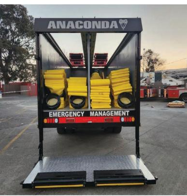
Anaconda has given us insight into the importance of the municipal market giving consideration to a large volume hose carrier for smaller diameter hoses (100mm/150mm) that can assist at an incident that requires extensive lengths of hoses to be laid and retrieved in a short space of time. Indeed,
