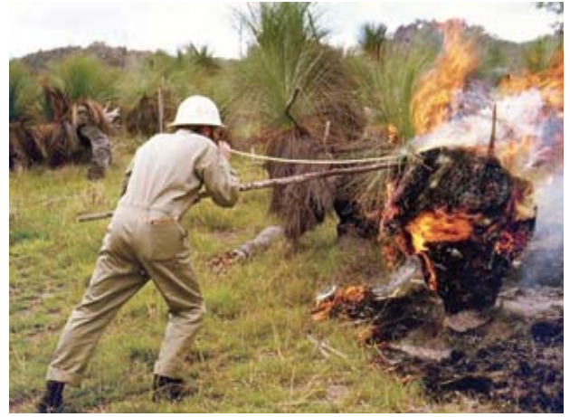
Sampling Smoke from burning Grass Tree to test for ethylene
