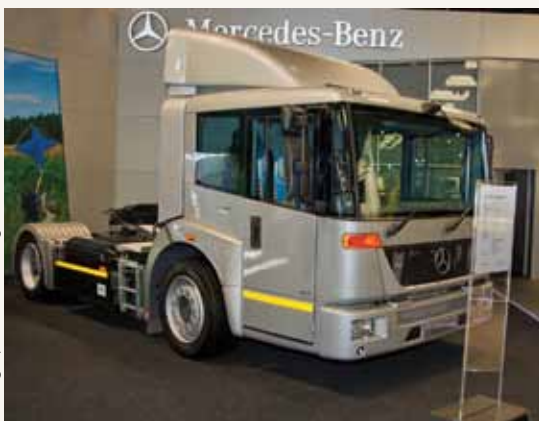
Mercedes Benz exhibited its 6-cylinder Econic 1828LS35 truck tractor that boasts a compressed natural gas (CNG) drive system
