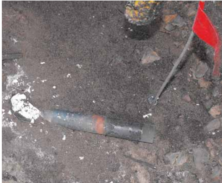
The handheld distress flare located some distance away that was the actual cause of the fire
