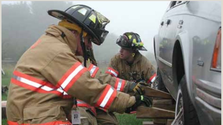
Wedges are extremely versatile and are used mostly to fill the spaces that are not in contact with the load or the ground
