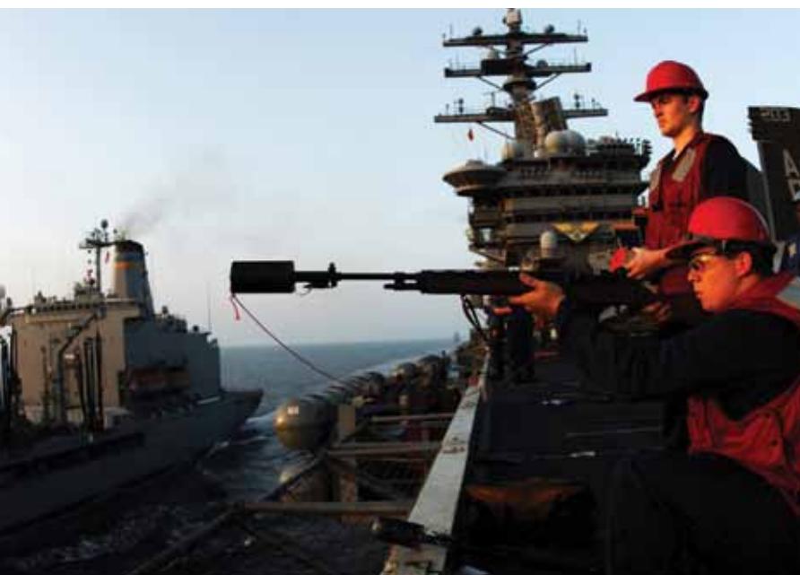
A line-thrower can be used in ship-to-ship line deployment
