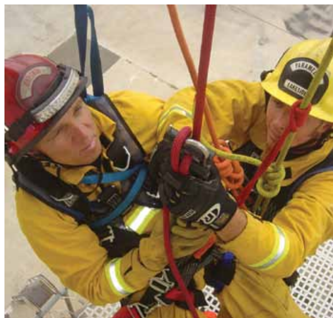
ResQmax may be used to establish the first vertical rescue line for rapid ascent rescuers
