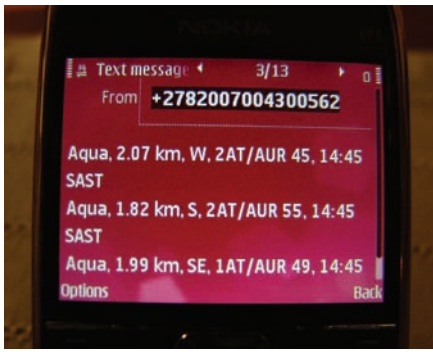
Figure 3. An example of three text message alerts of a fire received from the Aqua satellite. The first one is of a fire 2,7km west of tower 45 on the No2 Ankerlig – Aurora line. The observation time was 14:45 South African Standard time.
