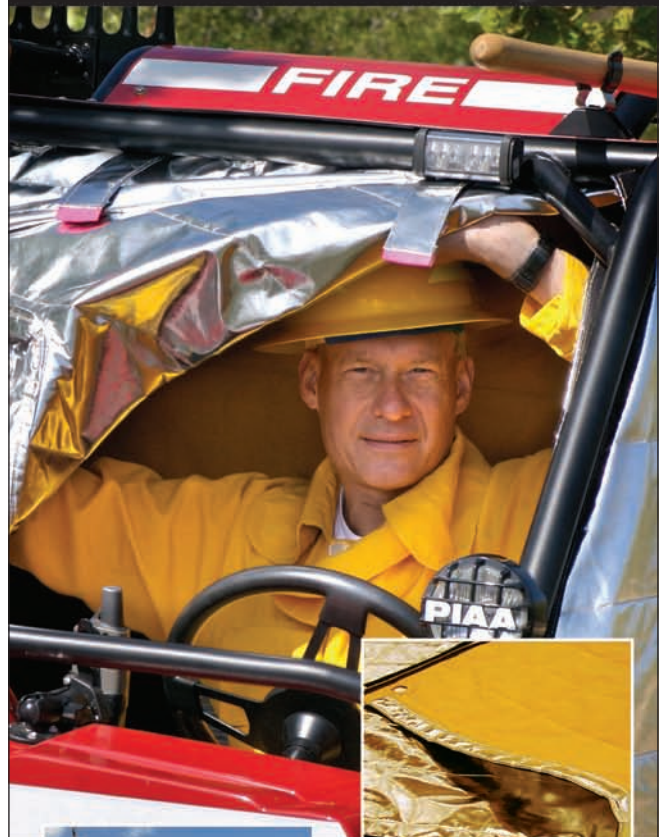
Storm King Mountain fire barrier shield, with reflective outer and yellow Nomex inner sides tested and approved by Country Fire Authority, Storm King Mountain material P/N 15302-101.
