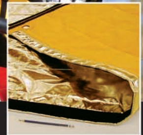
Storm King Mountain fire barrier shield, with reflective outer and yellow Nomex inner sides tested and approved by Country Fire Authority, Storm King Mountain material P/N 15302-101.
