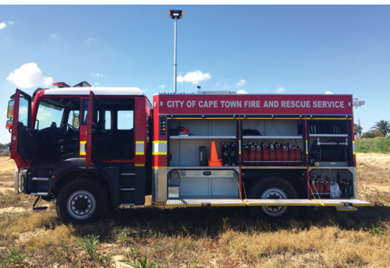
The flip-down locker doors below the mid-level lockers and wheel arches form a solid walkway along the sides for access to top shelves
