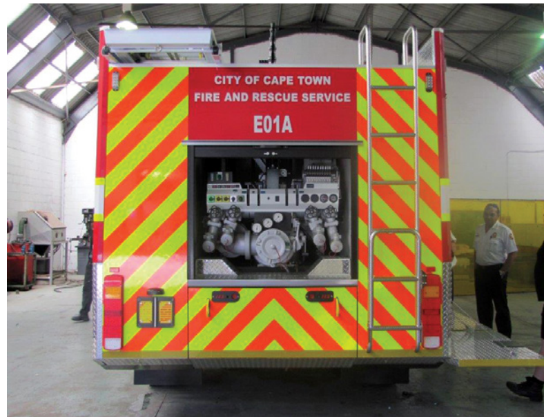
The Rosenbauer NH40 pump delivers 4 000l/min at 10 bar normal pressure and 45 bar high pressure
