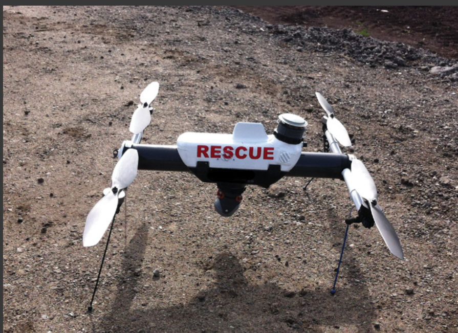
AeroVironment's Qube drone can hover and transmit live video and metadata to a tablet controller as part of search and rescue operations
