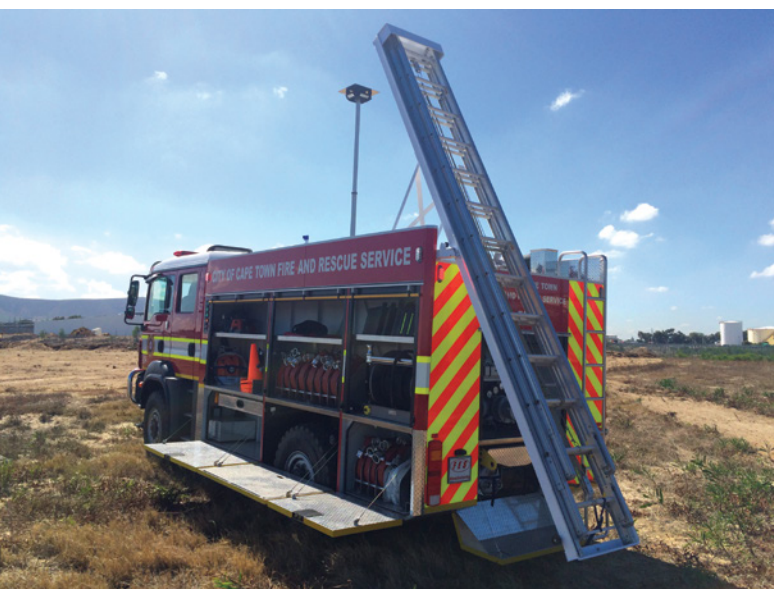
The single operator ladder gantry and triple extension ladder on the vehicle deck
