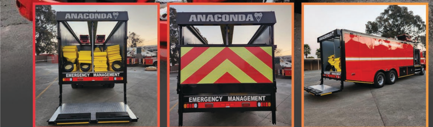
An automated large volume hose retrieval vehicle for retrieving hoses from 6" to 12"
