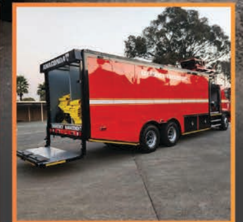
The unit is fitted with a dual Hose Mule System that automatically retrieves and flakes hoses
