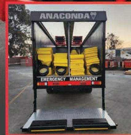
An automated large volume hose retrieval vehicle for retrieving hoses from 6" to 12"
