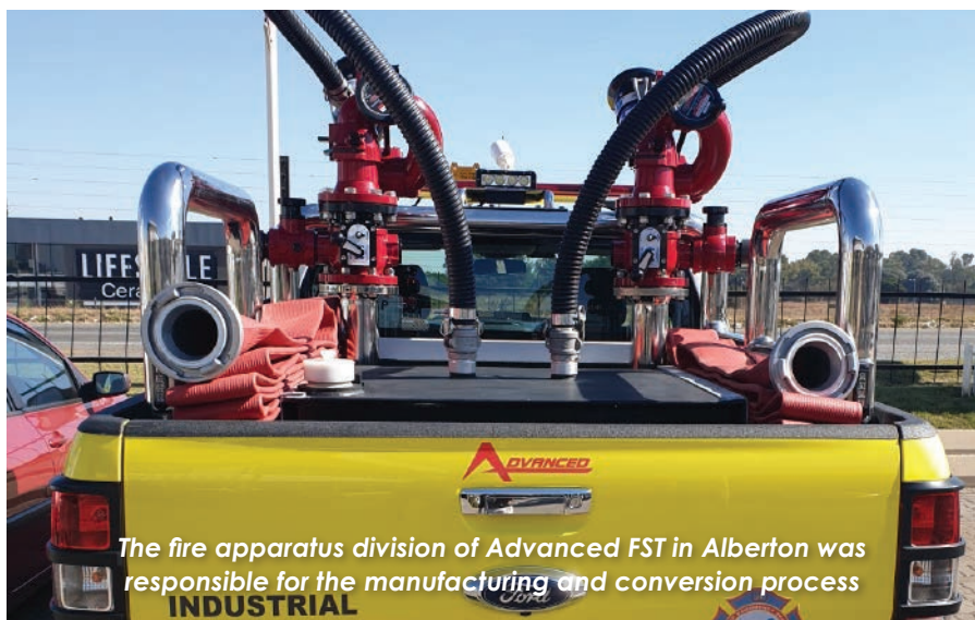
Two T-Series Crossfire monitors has been fitted with a T-Series Master Foam self-inducing nozzle
