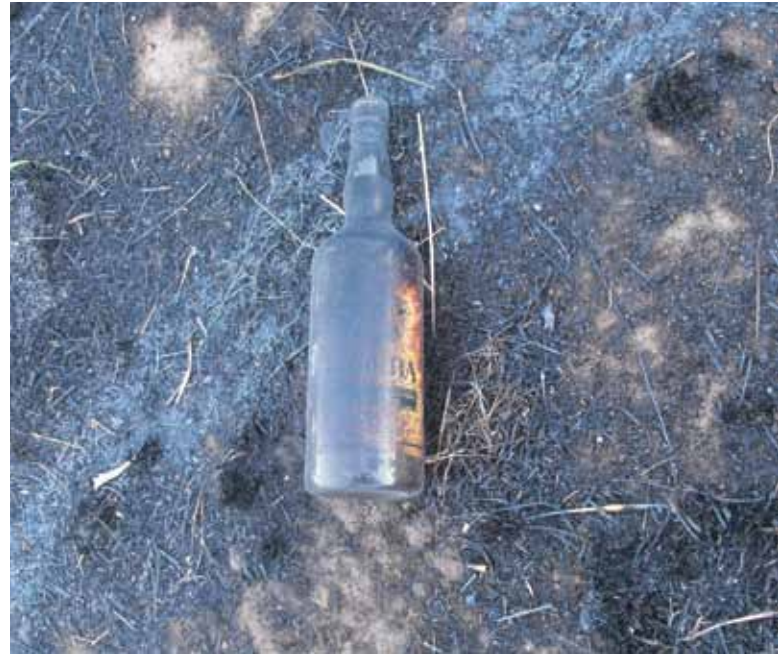
In above photograph the fire came from the left as can be seen by the black sooting on the bottle, as well as the grass stubble to the right that was protected by the bottle from the flames
