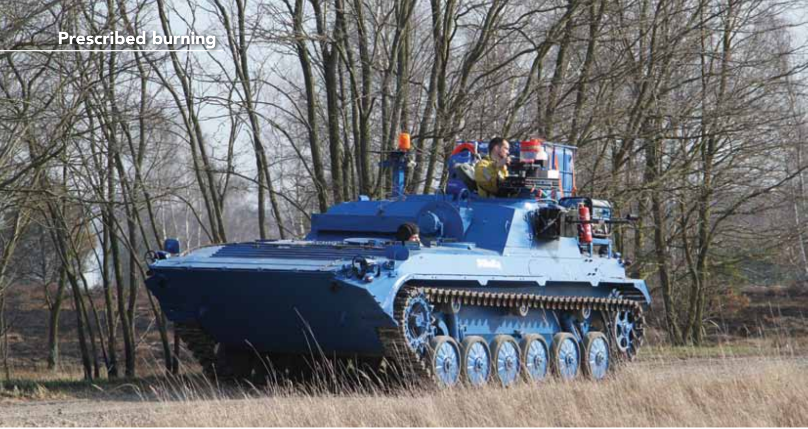
Ignition with the Russian BMP light tank fitted with a Green Dragon incendiary device
