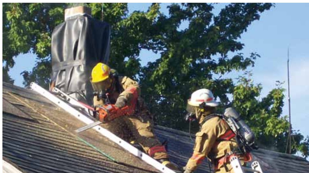
Ladders should provide quick and safe access to the roof, safer footing for any pitched roof and spread the load imposed by the fire fighters
