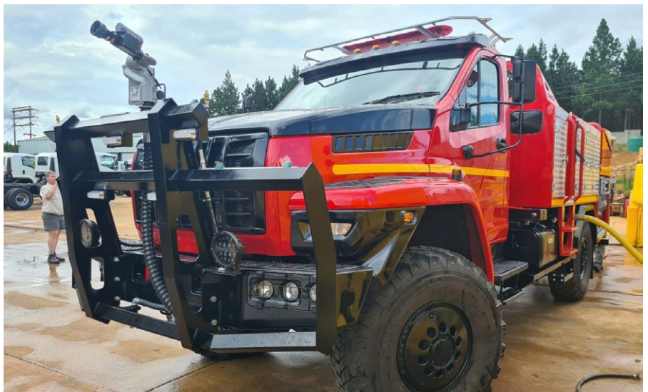
The new Anco fire engine was built on a Ural 43-206 4x4 chassis cab
